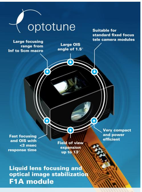
Our ultra compact F1A module enables four functions in one, namely focusing, macro, optical image stabilization, and field of view expansion.
