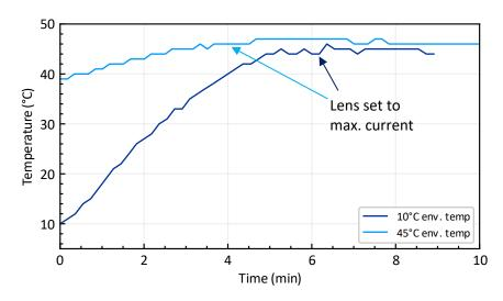
Figure 6: Initial heating phase for two extreme environmental temperatures 10°C and 40°C.
