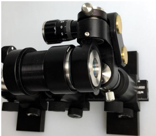
Figure 6: Example of mechanical mounting of the tunable prism with standard off-the shelf components and 2 adapter rings.
