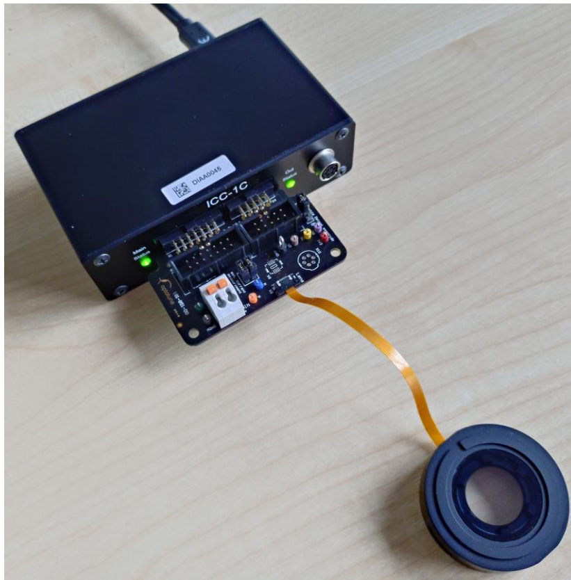
Figure 6: Connecting to a lens with FPC connector
