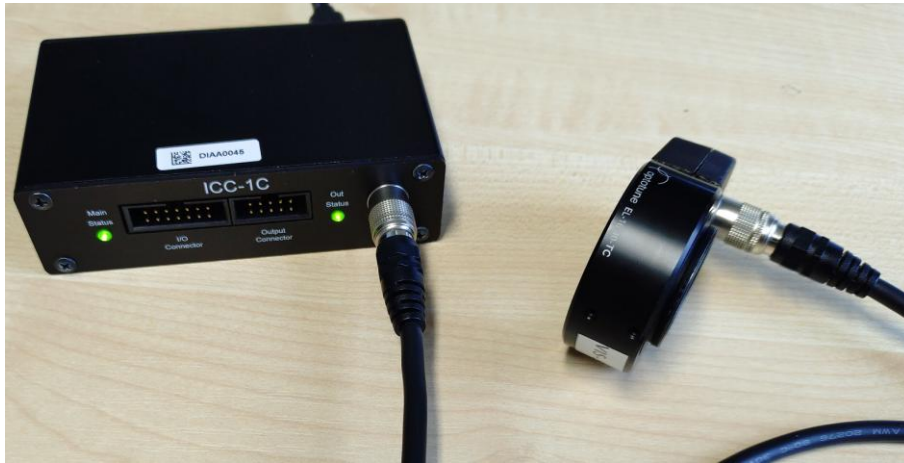
Figure 5: Connecting to a lens with Hirose connector
