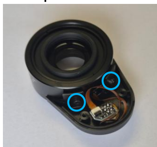
Unscrew the bottom adapter part with 1.5mm Allen key
