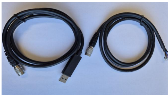
Figure 5: USB to UART and Hirose to open-ended wire
