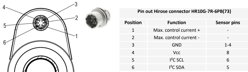
Figure 4: Electrical connections of lens models without embedded controller featuring (male) Hirose connector.
