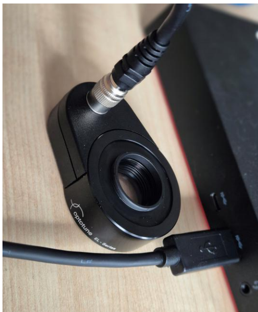
Figure 10: ECC-1C connected to USB interface
