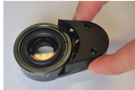
Remove the adapter by lifting it from the side
