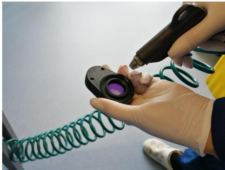
Figure 4: Dust-Cleaning of the EL-16-40-TC with adapter.
